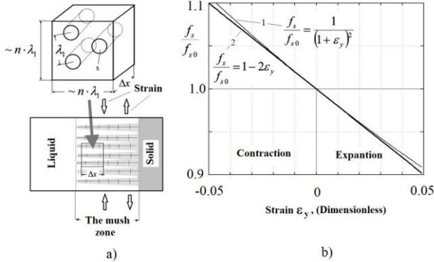
Fig. 2. Deformation effect on solid fraction variation in the mushy zone. a) Schematic diagram of a small volume element with a perpendicular section to primary dendrite arms in the mushy zone, b) Solid fraction variation as a function of relative deformation computed by a more (1) and less (2) exact formulas
