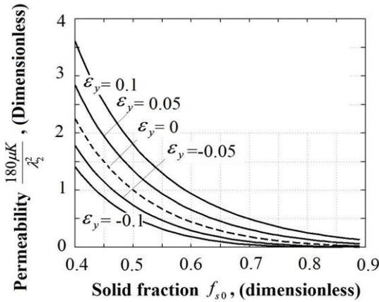
Fig. 4. Deformation effect on the permeability coefficient in the mushy zone. Hydraulic permeability versus solid fraction in the absence of deformation is shown with a dashed curve.
