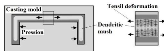
Fig. 1. Appearance of tensile deformation in the casting mushy zone under hindered shrinkage
