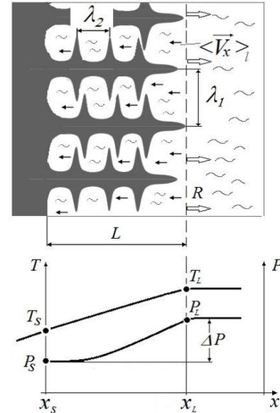
Fig. 3. Filtration model and schematic diagram of temperature and pressure fields over the mushy zone width
