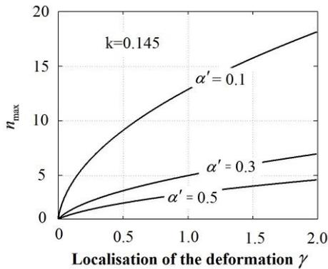
Fig. 6. Maximum deformation effect factor versus coefficient of deformation localization
